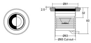
Soft silicon seal holds the fitting into the cut-out
